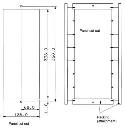
CAUTION Attach packings (acrylonitrile-butadiene rubber, or soft NBR) to prevent the ingress of oil and dust.
