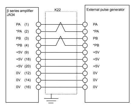
Connector : FI40-2015S (Hirose Electric) Case : FI-20-CV (Hirose Electric)
