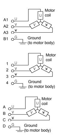
The standard receptacle connectors for models  $\beta 1$  to  $\beta 6$  do not exactly satisfy the MS standard in that the connectors are waterproof as single units, and their exterior color is black. However, their sizes and shapes are compatible with the conventional round-type connectors conforming to the MS standard.
