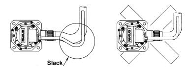
(c) When the motor connector is up, the cutting fluid is collected in the cable connector through the cable. Turn the motor connector sideways or downward as far as possible. Most of the defects caused by the cutting fluid have occurred in the cable connector.
