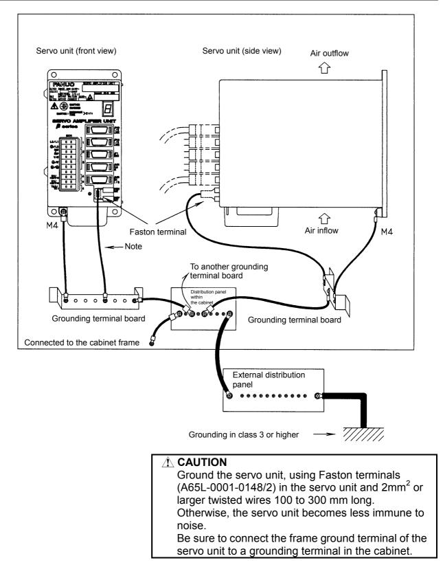
B-65232EN/03 FANUC AC SERVO AMPLIFIER β series 8. CAUTIONS FOR SAFETY STANDARDS RELATED TO AMPLIFIER INSTALLATION
