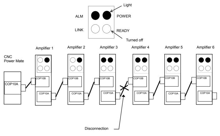
When the optical cable connecting the third  $\beta$  amplifier with the fourth  $\beta$  amplifier, the "ALM" LEDs on the third and subsequent amplifiers are turned on, and the "LINK" LEDs and the "READY" LEDs are turned off.
