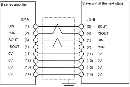
Specifications of a recommended connector and case for cable K20 on the  $\beta$  series amplifier side
