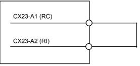
Cable specification : Vinyl cabtyre cable, JIS C 3312, 2 conductors Conductor 3.5 mm<sup>2</sup> Housing : 2-917807-2 Contact : 316041-2 Applicable power line range : 3.5mm<sup>2</sup> to 5.5mm<sup>2</sup> Manufacture : tyco Electronics AMP
