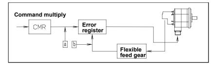
In the above figure, each ratio is set so that the units of the two inputs (a and b) of the error register are the same. The  $\beta$  pulse coder uses a flexible feed gear as standard. So, CMR is normally set to 1. When other than 1 is to be set for CMR, contact FANUC for details.
