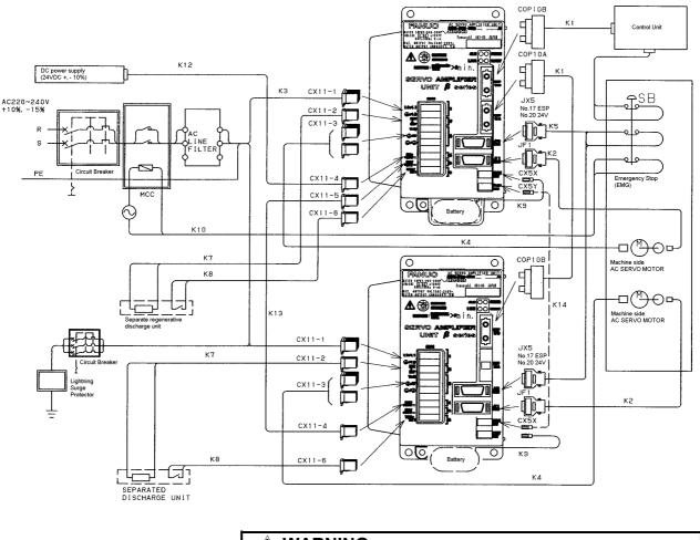
Be sure to install circuit breakers, magnetic contactors, and AC line filters.
