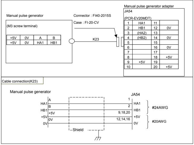
Recommended wire : A66L-0001-0286 (#20AWG  $\times$  6 + #24AWG  $\times$  3 pairs)
