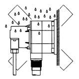
(b) Prevent the cutting fluid from being led to the motor through the cable. When the motor connector is used in the sideways position, put a drip loop in the cable.
