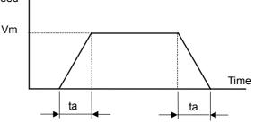
(h) Distance of positioning in rapid traverse Enter the amount of travel when positioning during rapid traverse.
