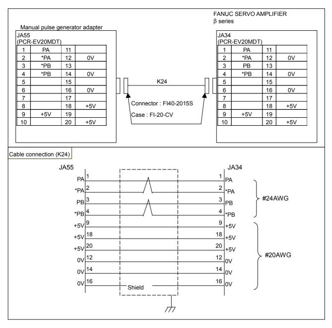
Recommended wire : A66L-0001-0286(#20AWG × 6 + #24AWG × ×3 pairs) Recommended connector : A02B-0120-K303 Maximum wire length : Up to 5 m
