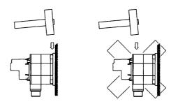
(5) When handling model  $\beta$ M0.2/4000 or  $\beta$ M0.3/4000, be sure to hold the main body of the motor. Do not carry the motor by holding the lead wire only.
