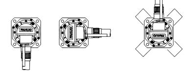
(d) The connectors and lead wires of power and signal lines of models  $\beta$ M0.2/4000 and  $\beta$ M0.3/4000 are not drip-proof. When a connector or lead wire must be drip-proof, the machine tool builder needs to provide drip protection.
