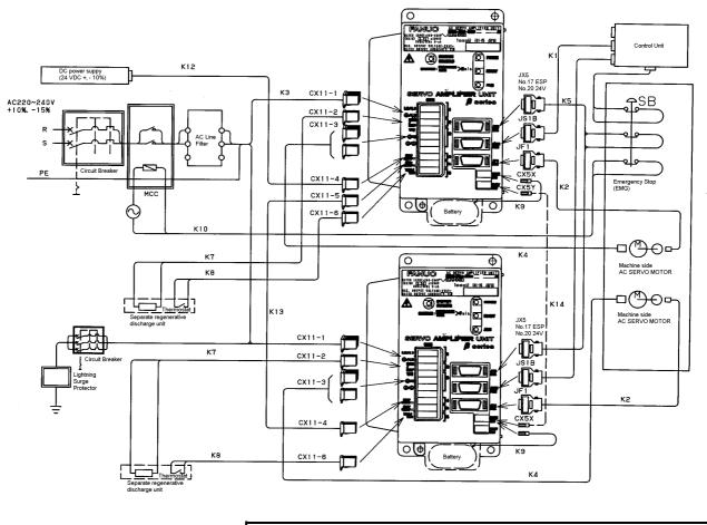
▲ WARNING Be sure to install circuit breakers, magnetic contactors, and AC line filters.
