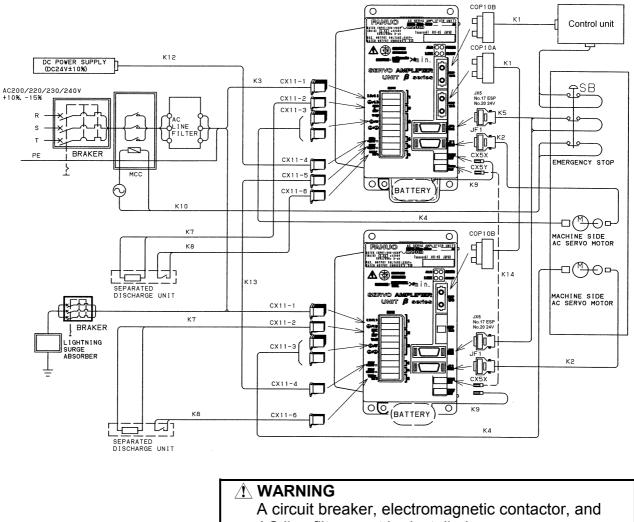
AC line filter must be installed.
