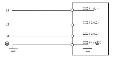
Housing : 1-179958-4 Contact : 316041.2 Applicable power line range : 3.50mm<sup>2</sup> to 5.50mm<sup>2</sup> Manufacturer : tyco Electronics AMP Wire to be used 600V vinyl cabtyre cable, 4 conductors (Nominal sectional area : 3.5 mm<sup>2</sup>)
