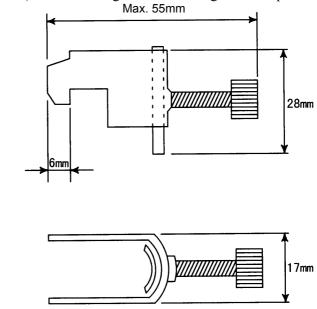
Fig.7.3.4(e) Outer drawings of metal fittings for clamp
