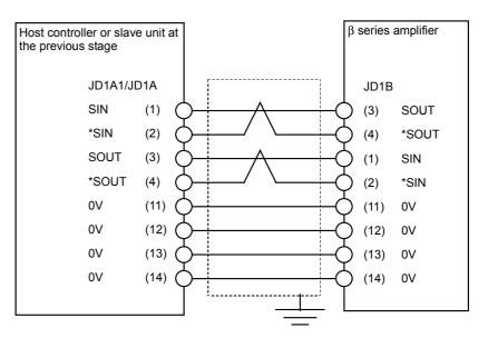
Details of connection of cable K20 (when a connection is made with the host controller or the slave unit at the previous stage)
